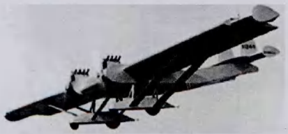
图1 伯内利采用伸缩机翼设计的GX-3飞机 Fig.1 GX-3 aircraft with telescopic wing designed by Burnelli
